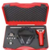
Acoustic leak detection of heating installations
