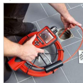
Inspection of floor drains
