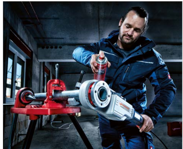
Die heads with the tripod universal workbench
