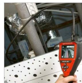
Camera head with high-performance LEDs
