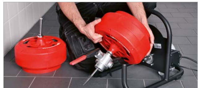
Interchangeable drum for different working ranges
