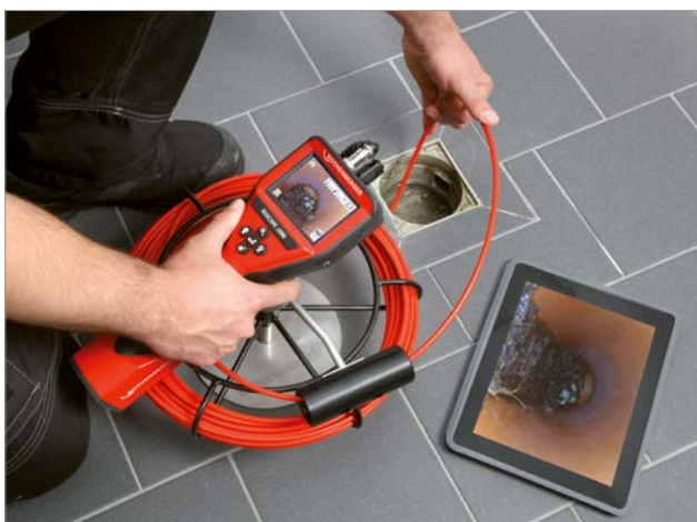
Inspection of basin drains
