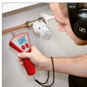
Acoustic leak detection of heating installations
