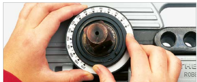
Pre-adjustment of the bending angle without tools
